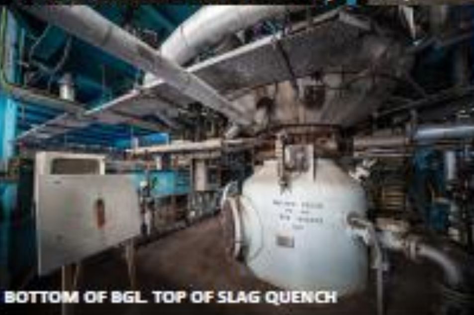
STEAM & OXYGEN INJECTION NOZZLES (TUYERES)
